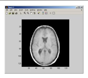
We apply ConfidenceConnectedImageFilter to the resulting filtered image. The following example illustrates how the seed point (102, 82, 25) is supplied as an argument:
