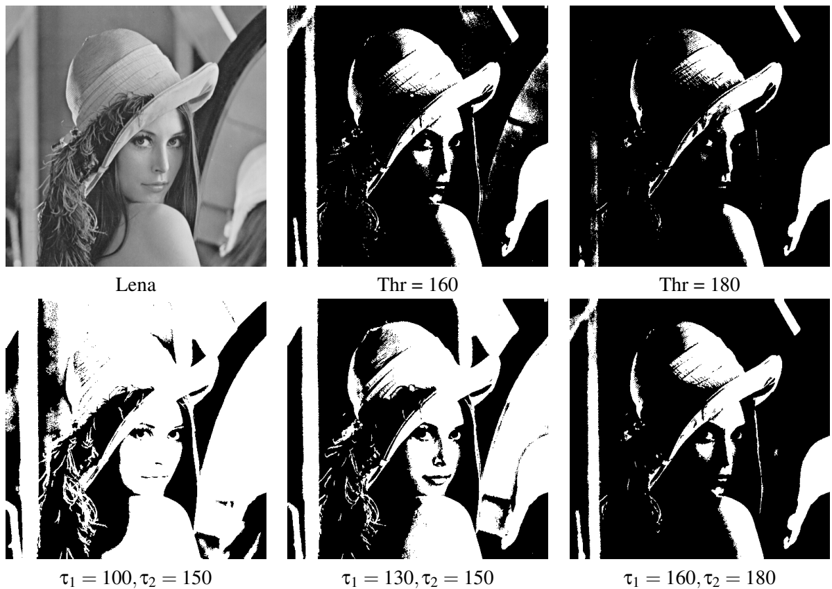
Figure 1: Example of hysteresis thresholding and ordinary thresholded using the classic Lena image. Upper row, original image and standard thresholding. Bottom row, thresholds with hysteresis.
