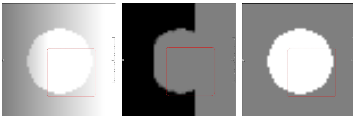
Figure 2: (a) original image in 2D (b) segmentation using Chan-Vase in 2D contour (c) segmentation using RSF in 2D. The red contour shows the initialization.
